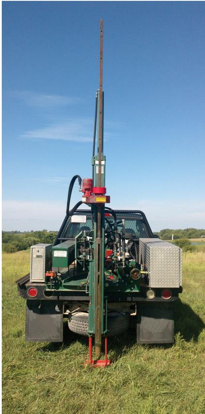
*A truck-mounted hydraulic probe used to quickly obtain soil profiles. The Giddings probe (shown) has the ability to collect a large- or small-diameter core sample, and extensions can be added to it for deep coring. Driver's side-mounted bull probes are preferred in some areas but are limited to collection of smaller diameter core samples. (Photo courtesy of Casey Latta)*
